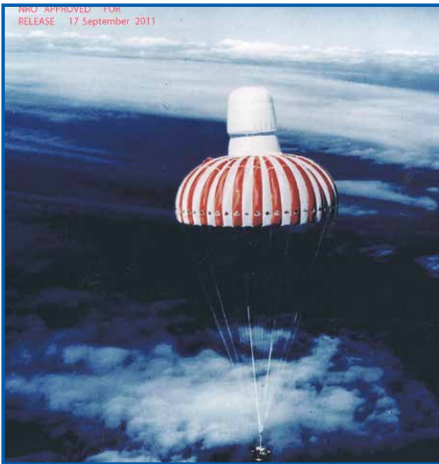
Figure 16: KH-9 HEXAGON Mark 8 “extended skirt” parachute with bucket below.
