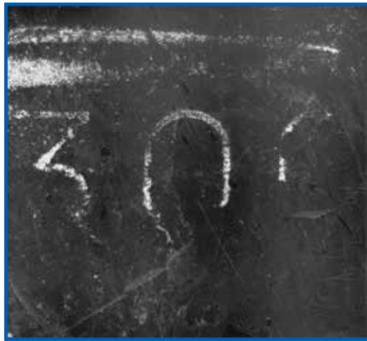
Figure 15: Photo taken during Eastman Kodak's post-salvage analysis of recovered film shreds showing the number 300 imprinted on the film. Paint transfer due to the extreme impact shock caused the imprint. Credit: CIA
